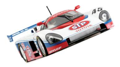
The car, designed by Dome, was an evolution of the 87 model. It was powered by a 2.1 litre, water cooled, 680-hp, 4 cylinder turbocharged engine unit, named "3S-GT", with 16 valves driven by double over head camshaft.
