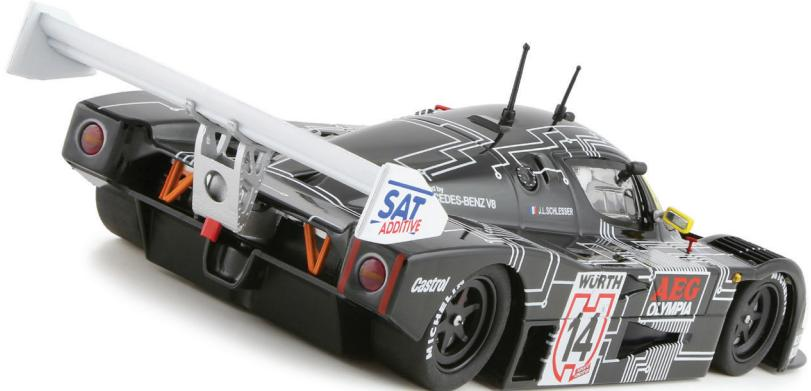
Chassis was mainly an aluminium monocoque, with magnesium elements and carbon-fibre skins. It had double wishbone suspensions, with direct-action at front and rocker-arm at rear, as well as Speedline magnesium rims, 17" front and 19" rear, and Brembo cast-iron 14" disc brakes.
