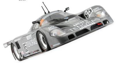
The car featured a kevlar and carbon-fibre based monocoque chassis fitted with Nissan's new twin-turbo VRH35 3.5L V8 DOHC engine which was mounted in a stressed installation for better chassis rigidity, delivering up to 950bhp.
