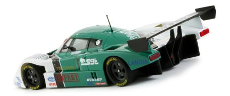
Chassis was made of aluminium and magnesium while body was carbon fibre composite. The overall weight was 850 kg. Lancia LC2s were as quick as Porsches, in terms of pure speed, but lacked reliability.
