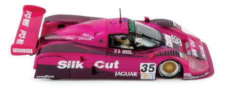
This model featured a carbon fiber monocoque chassis. The engine was a V12 engine with two valves per cylinder. In 1990, displacement was 6 liters for the IMSA version and 7 liters in the Group C configuration; these values were increased in 1991, becoming 6.5 liters for the American version and 7.4 for the European one, whose weight was respectively 930 and 1000 kg.
