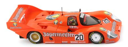
The Porsche 956 and later 962 models could be assembled with two different rear wing configurations: "low downforce", used mostly in Le Mans where the 6.5 km Hunaudières straight required a very low drag at the expense of downforce, and "high downforce", for twistier circuits.
