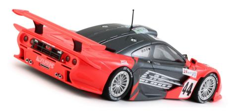
The car featured a monocoque carbon – fibre chassis and a BMW 5990 cc V12 engine.
