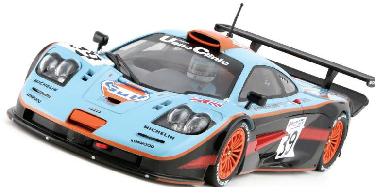
The car featured a monocoque carbon - fibre chassis and a BMW 5990 cc V12 engine.
