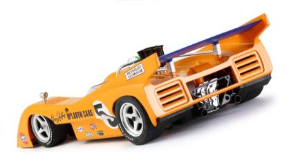
The M8D was a prototype race car, built in 1970 by McLaren Cars to compete in che Can-Am Challenge Cup. In comparison with the former 'M8', the M8D was wider and with a lower wing, which was also braced to the chassis, as the high mounted, suspension attached wings had been banned. Chassis was an aluminium sheet monocoque with steel bulkheads and stressed engine. Bodywork was in glass-fibre.
