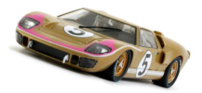
Visually, the MKII wasn't too different from the MKI. Its distinctive characteristics were the rear bonnet and the engine: the new, big, V8 had a displacement of 7.0 liters (427 ci); the power was 485 hp at 6300 rpm, and the car was able to reach a maximum speed of 330 km/h.
