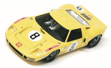
The GT40 was engaged among the "Sport" cars, with a road homologation and a limit of 5 liters for displacement. The chassis was a steel semi - monocoque, the body was made of fiberglass.
