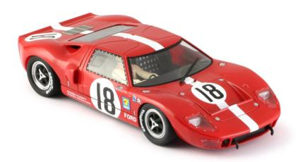
The chassis was a steel semi - monocoque, the body was made of fiberglass. The engine came from the one used on the AC Cobra, with cast-iron block and head: naturally aspired V8, 4.7 litres displacement, 2 valves per cylinder operated by a central camshaft with push-rod; it was coupled with a ZF 5 speeds gearbox. Brakes were provided with vented discs on all the four wheels.
