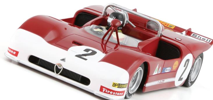
The 'T33/3' cars featured a monocoque chassis, paneled in aluminium and magnesium, a V8 2998 cc engine, and a 6 or 5 speed gearbox. Top speed reached 330 km/h, at Le Mans with long tail.
