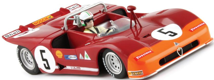
The 'T33/3' cars featured a monocoque chassis, paneled in aluminium and magnesium, a V8 2998 cc engine, and a 6 or 5 speed gearbox.
