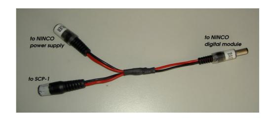
Plug the black cable from the SCP-1 cartridge (SCP01e) to the NINCO digital module and run.
