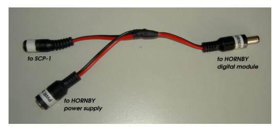
Plug the black cable from the SCP-1 cartridge (SCP01e) to the HORNBY digital module and run.
