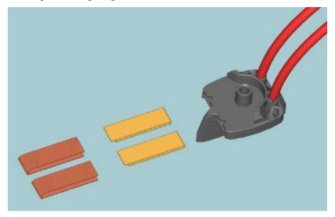
3. insert the brass tabs (and the braid they are wrapped around to) in the pickup
