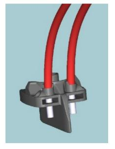
2. bend the brass tabs following the pre-etched middle line, and wrap them around the braid. Keep the longest part of the tab UP.
