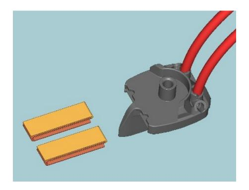
4. press the tabs all the way until they are aligned with the pickup edges. Trim off extra wire from the rear end of the pickup.
